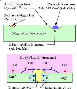
In Mg alloys, Pitting corrosion occur at free corrosion potential of magnesium, when exposed to chloride ions in a non-oxidizing medium. The as-extruded magnesium alloy AM60 was immersed in natural 3.5% NaCl solution, and the corrosion pits occurred on the surrounding of AlMn particles. The alloy has a protective oxide film in air. The potential of MgO (+1V), when it is immersed in a sodium chloride aqueous solution, C1- ions will absorb on the  $\alpha$ -Mn areas bordering on Al-Mn particles.
